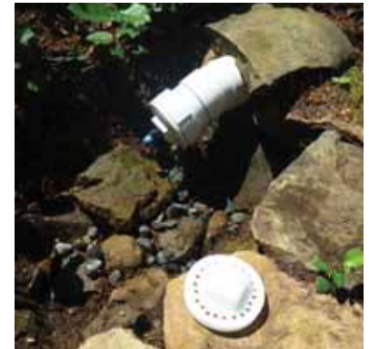
FFD dripper end and plug with many holes.
